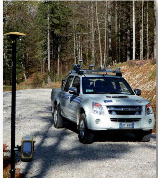
The implementation of the Mobile Mapping System developed by Siteco, allowed the region department staff to carry out a mobile survey, with accuracies that ranged from a few centimeters (in the case of ordinary roads with a good GNSS signal), to sub metric values (in the case of forest tracks where the GNSS signal was absent even for several minutes).
