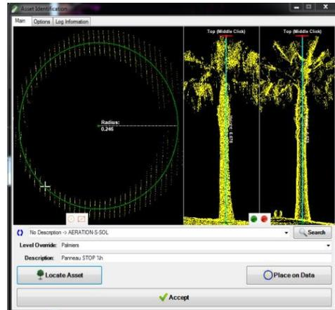
FIGURE 7. PALM TREE EXTRACTION IN TOPODOT USING HORIZONTAL AND VERTICAL SECTIONS
