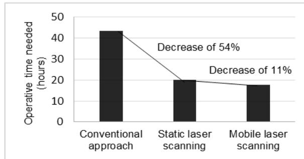
FIGURE 13. OPERATIVE TIME NEEDED FOR EACH METHOD TO ESTABLISH AN URBAN SURVEY FOR A SECTION OF 300 METERS LENGTH (SCALE 1:200)
