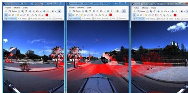
FIGURE 4. VIDEO IMAGES OVERLAY WITH POINT CLOUD VISUALIZED IN ROADSIIT SOFTWARE
