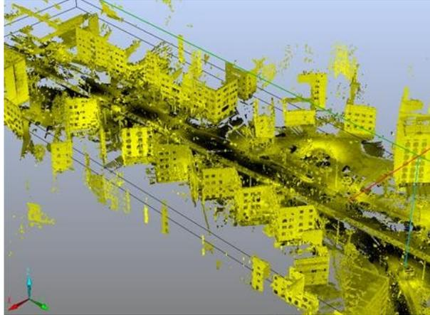
FIGURE 2. 3D VIEW OF FINAL POINT CLOUD RESULTING FROM STATIC SCANS
