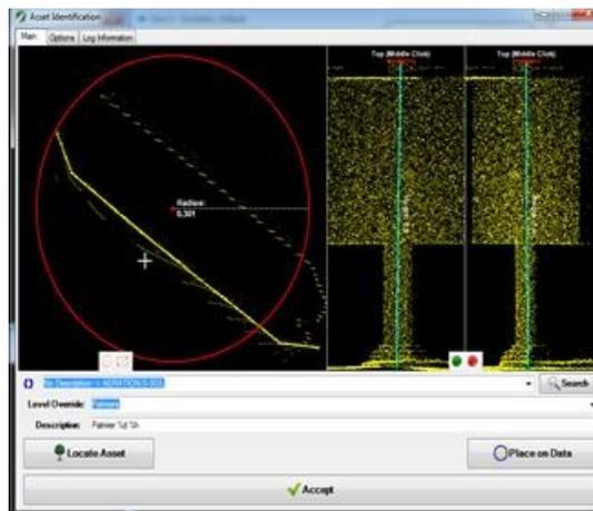
FIGURE 8. AN ADVERTISING PANEL EXTRACTION EXAMPLE USING TOPODOT
